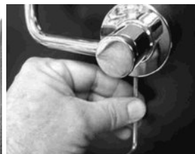
Tighten or remove using Allen Key
